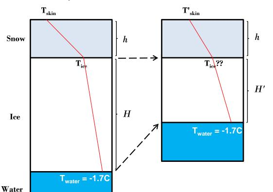
$$k_{ice} \frac{\partial T_{ice}}{\partial z} = k_{snow} \frac{\partial T_{snow}}{\partial z}$$
